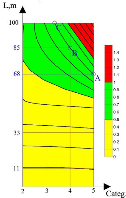
**Fig. 6.** Dependency of accuracy of point heights obtained from DTM on density of regular grid and on complexity of relief
