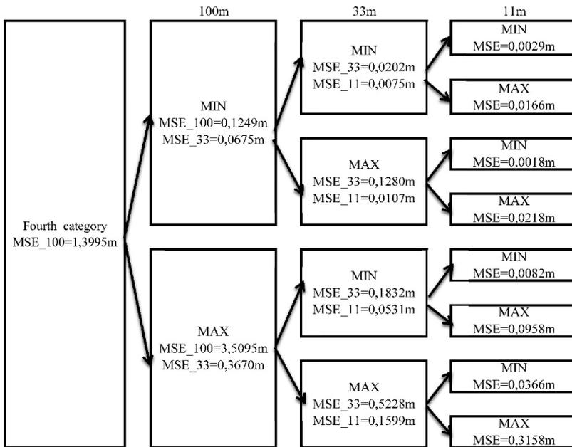
Fig. 4. Results of accuracy estimation of DTM reconstruction at thickening a regular grid (fourth category of complexity)
