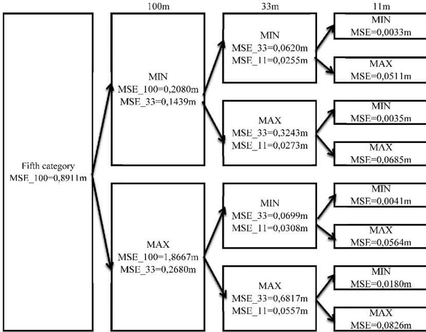
Fig. 5. Results of accuracy estimation of DTM reconstruction at thickening a regular grid (fifth category of complexity)
