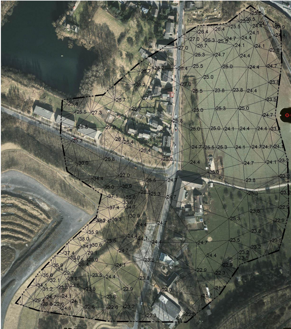
Fig. 11. Land plot physical area modeling using TIN model
