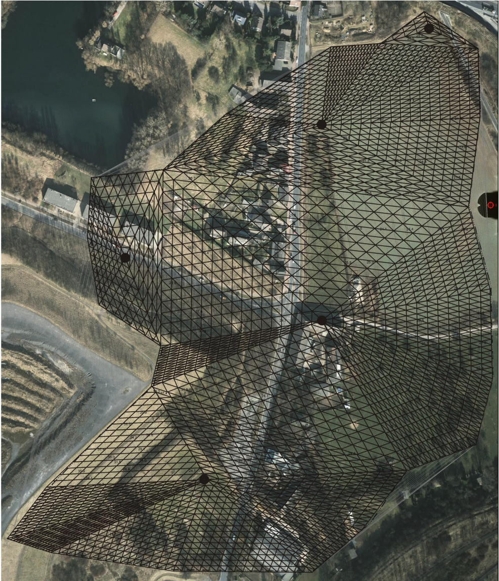
Fig. 13. Land plot physical surface modeling by developed methodology
