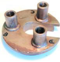
Fig. 7. Handle transferring force to foundation (top)
