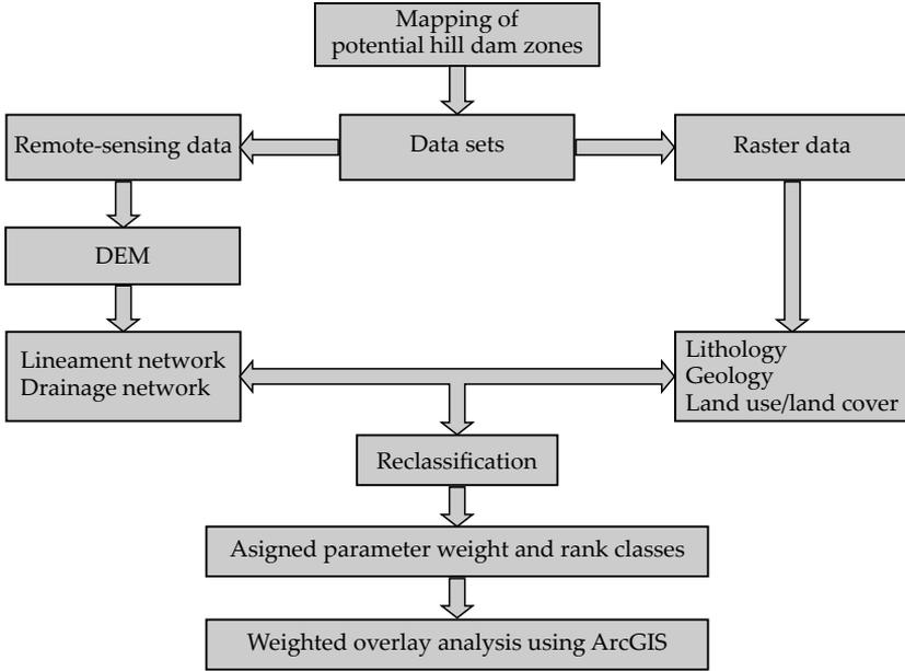
Fig. 3. Flow chart that illustrates step-by-step process of mapping potential areas for hill dam planning
