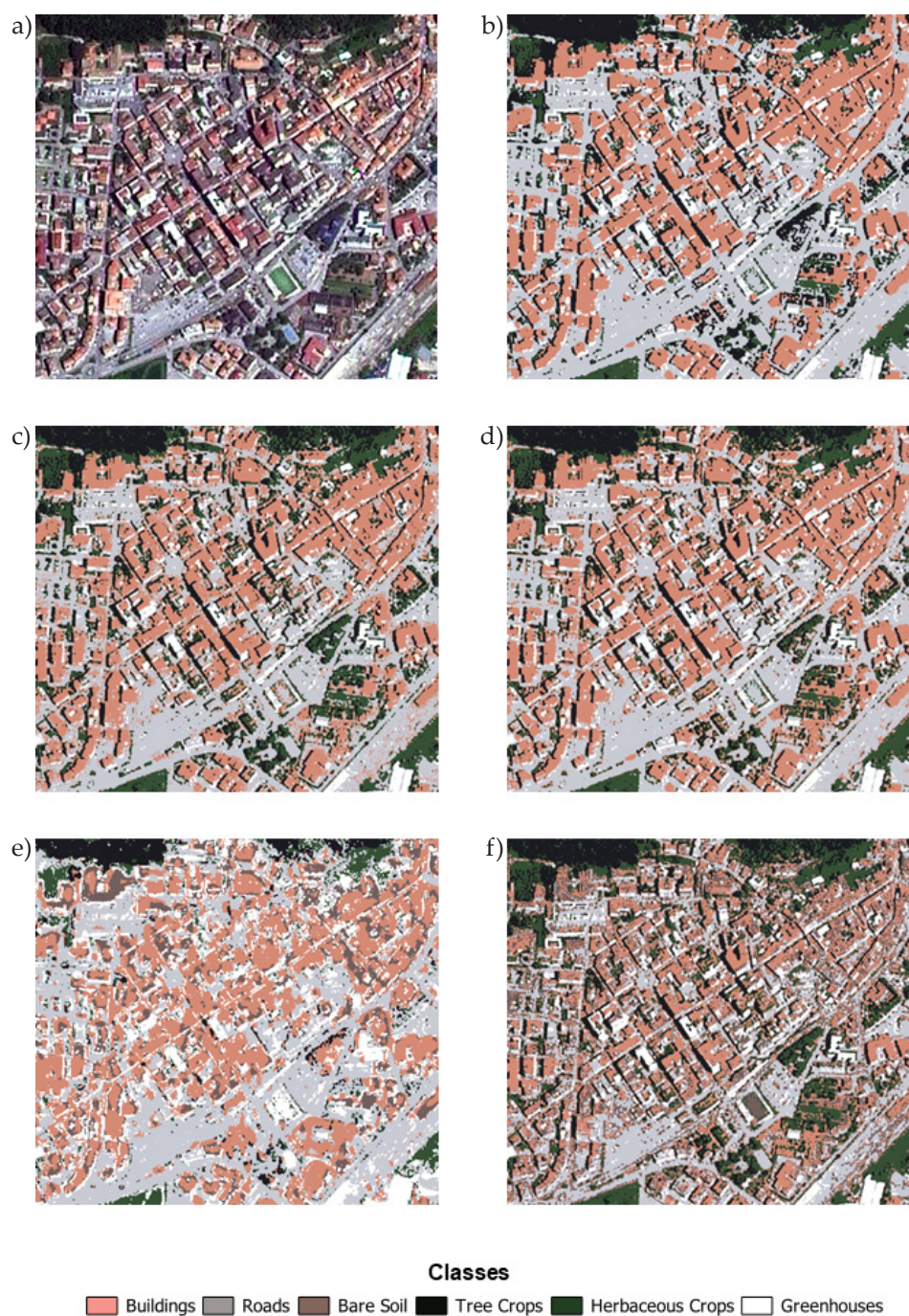
Fig. 7. Zoom-in on small portion of study area to graphically show classification results for RGB composition (a) by following methods: SVM (b), DT (c), k-NN (d), NB (e), and RF (f)
